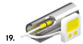
19. EC testing of inner surfaces
